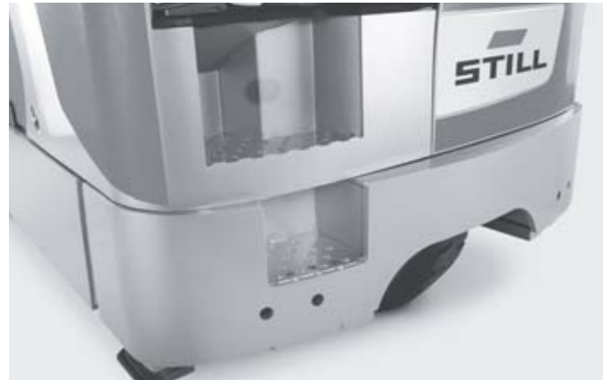
Safe entry thanks to additional step
